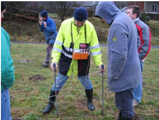
Reducing the space between the checkpoints the mistake can be localized with accuracy less than ca 2cm!!
