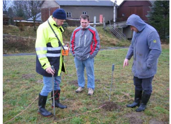
Giving HV- impulses at the line, the difference between two points can be measured!
