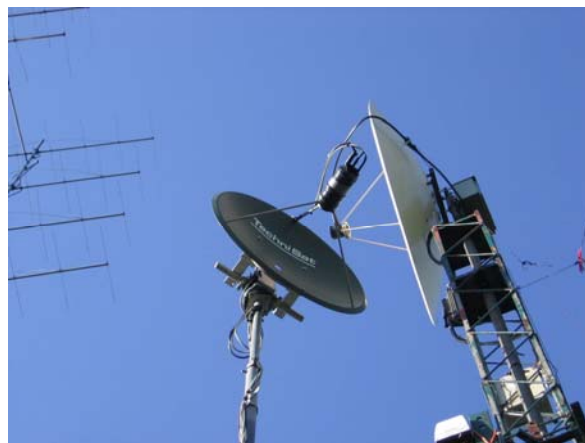
Last not least the used antennas, left the 90cm dish for 10368MHz, right hand the 1.5m dish for 2320MHz
